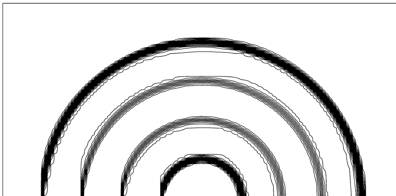
Fig. 13. Step test case – scalar contours for Superbee scheme.
